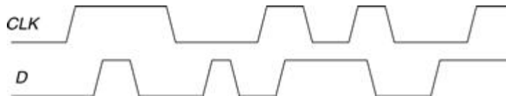
Figure 3.63 Input waveforms of D latch or flip-flop for Exercises 3.3 and 3.5
