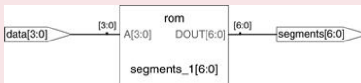
Figure 4.20 sevenseg synthesized circuit
