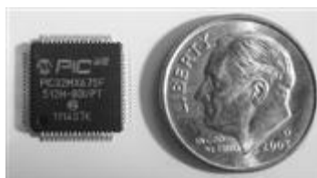
Figure 8.32 PIC32 in 64-pin TQFP package
