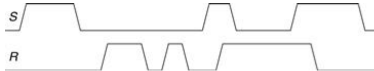
Figure 3.61 Input waveforms of SR latch for Exercise 3.1
