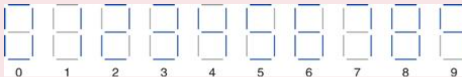
Figure 2.48 Seven-segment display digits
