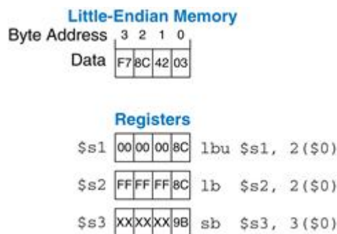
Figure 6.22 Instructions for loading and storing bytes
