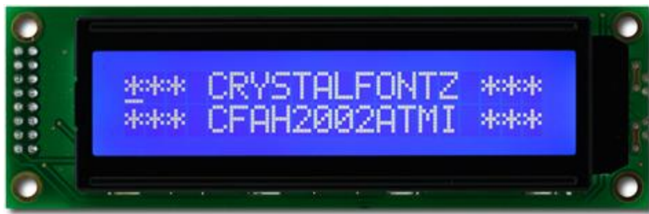
Figure 8.49 Crystalfontz CFAH2002A-TMI 20 \times 2 character LCD
